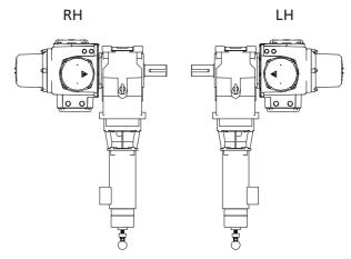
Figure 2.1. Left and right hand mounting orientation.
