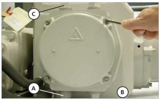
Figure 3.1. Terminal compartment cover
