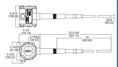
The **SERIES CLS2** Capacitive Level Switches is a capacitive technology level switch which can be used for liquids, powders and bulk materials. It is offered with PVDF and 316 SS wetted material, weatherproof enclosure, DPDT output and a variety of process connections
