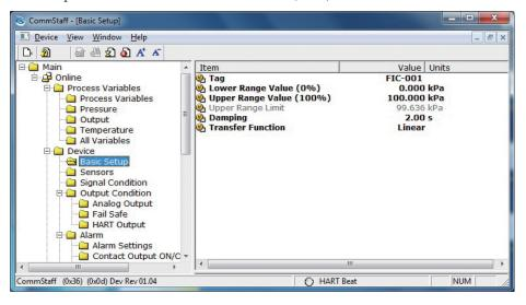
To change the setting for Upper Range Value (100 %), double-click that item in the right pane as shown above. A window opens for changing the setting. Enter the desired value and then click the Set button. Input the setting after deletion of the former setting.
