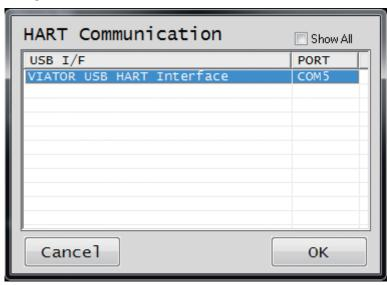
Note: If the desired COM port is not displayed, put a check in the [Show All] check box.
