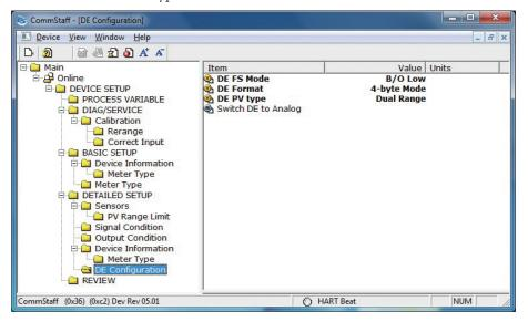
To change from DE Mode to Analog Mode (4–20 mA mode), execute the "Switch DE to Analog" method. After the changeover, the following screen is displayed. Be sure to exit CommStaff and restart it.
