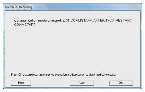
To change from Analog Mode (4–20 mA mode) to DE Mode, execute "Switch Analog to DE." In this case also, after the changeover, be sure to exit CommStaff and restart it.
