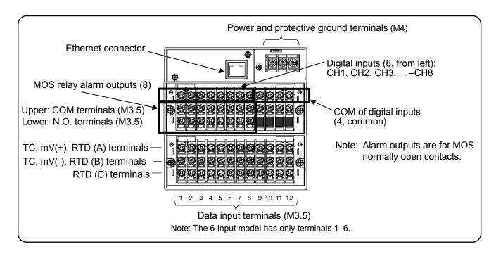
Note: The upper terminal block (including the alarm terminal block and the contact input terminal block) is removable for easy connection. Because the terminal block is connected by connectors, it can be removed easily by loosening two screws.
