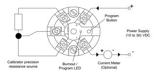
Figure 3 Configuration circuit
