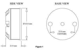
Mounting holes: two holes 5.5 mm diameter, 33 mm centers Center Hole sensor wire entry: 4 mm
