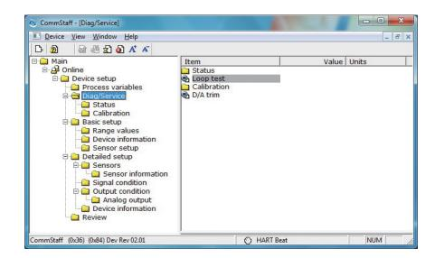
Double-clicking Loop Test displays the following screen.
