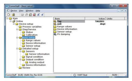
Double-clicking Tag displays the settings screen. On this screen, set the Tag and click the Set button. The tag is highlighted in yellow. Click the Send button to send the new Tag to the transmitter.
