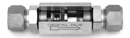
The **Tubing Check (TV)** valve is constructed with compression tube fittings (flareless) and is designed for a minimum pressure drop. The valves are furnished complete with ferrules and nuts. The TV valve can also be used as a low pressure relief valve or vacuum breaker by using the desired spring settings.
