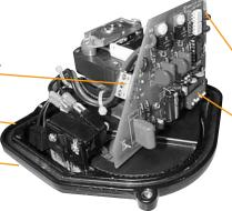
**Solid-State Timer** – provides reliable operation and low power consumption. Eliminates troublesome cams and mechanical switches.
