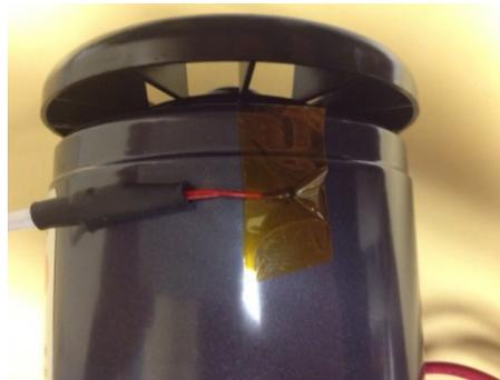
The red tip of the Thermistor must touch the outside of the motor housing. We recommend using high temperature tape to hold the tip to the surface.
