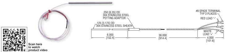
Precision **SERIES RTD** (Resistance Temperature Detector) offers excellent accuracy and stability over a wide temperature range. Industry standard 3-wire 100  $\Omega$  (DIN) probes are available in 6" (15 cm), 12" (30.5 cm), or 18" (46 cm) sheath lengths with 30" (76 cm) extension cable and spade lug terminals.
