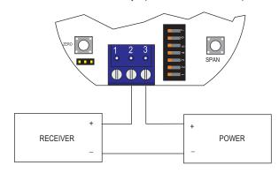
CURRENT OUTPUT WIRING Figure 2 The range of appropriate receiver load resistances (RL) for the power supply voltage available is given by the formula listed below. Shielded 2-wire cable is recommended for control loop wiring. Ground the shield at the power supply end only.
