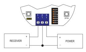
VOLTAGE OUTPUT WIRING
