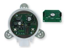
Another option for models that do not have a display would be to use a Model A-435-A remote display tool which can plug into the connector shown in Figure 7. The remote display tool has two buttons that function identically to the buttons on the PCB.
