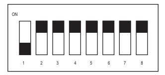
Figure 6: Address of transmitter is 127
