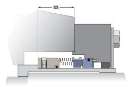
4.6 Tighten seal assembly set screws to shaft sleeve insuring seal assembly is retained at proper seal setting location as noted on seal assembly drawing.
