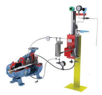
In some pressurized seal-system applications, pressure within the seal chamber varies, making it difficult to set the pressure for the barrier-fluid reservoir. The API Plan 53C tackles that challenge.
