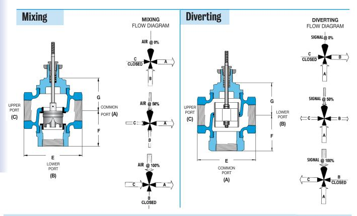
Trerice 3-Way Valves are not designed for use in steam applications.
