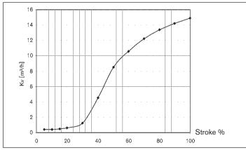
Fig. 5: Flow characteristics for orifice 25
