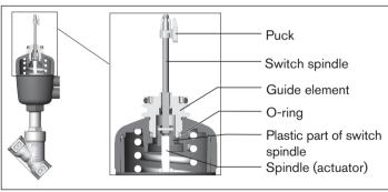
Fig. 13: Installing the switch spindle
