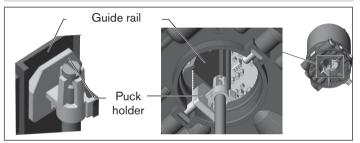
*Fig. 14: Aligning the puck*
