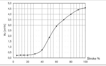
Fig. 3: Flow characteristics for orifice 15
