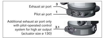
Fig. 17: Pneumatic connection
