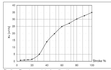
Fig. 7: Flow characteristics for orifice 40
