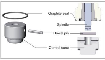
Fig. 19: Replace the control cone set
