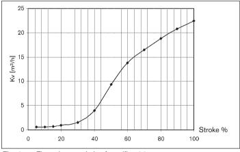
Flow characteristics for orifice 32 Fig. 6:
