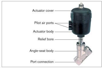
Fig. 1: Angle-seat control valve Type 2702, structure and description
