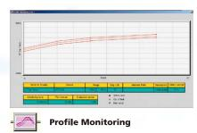
When a condition changes or the temperature for a batch operation is being controlled by programs, this icon is used to monitor whether the process value is moving on the assumed track.
