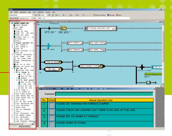
In the Explorer window, you can hierarchically organize an entire process and monitor it from a bird's-eye view. If anything abnormal occurs in the process, the symbol for the process changes color. From the symbol, the operator can directly call up the process in which the abnormality occurred.
