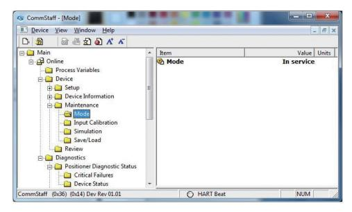
• When the Smart Positioner's power is turned on, it will go into In Service Mode.
