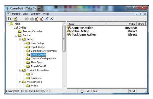
• Select Direct or Reverse for Actuator Action, Valve Action, and Positioner Action.
