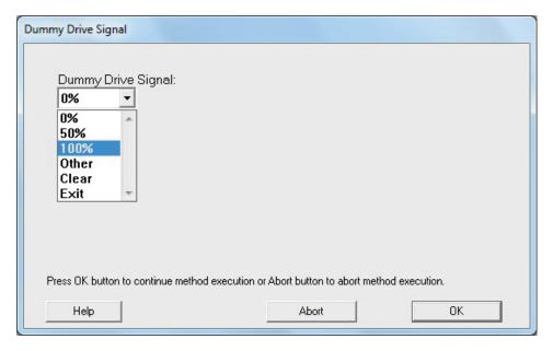
Selecting 0 % and clicking OK will keep the dummy EPM drive signal at 0 %.
