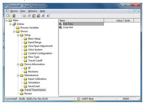
Connect the ammeter and calibrate the degree of opening transmission output for 4 and 20 mA.
