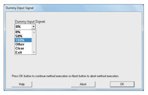
Selecting 0 % and clicking OK will keep the dummy input signal at 0 %.
