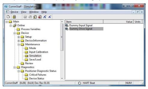
Make sure that the loop is set to manual and configure the dummy EPM drive signal in the window shown below.
