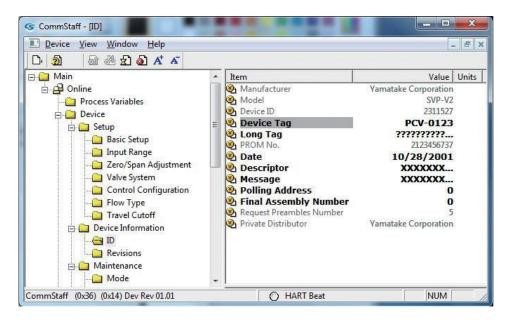
Double-clicking Tag displays the settings screen. On this screen, set the Tag and click the Set button. The tag is highlighted in yellow. Click the Send button to send the new Tag to the transmitter.
