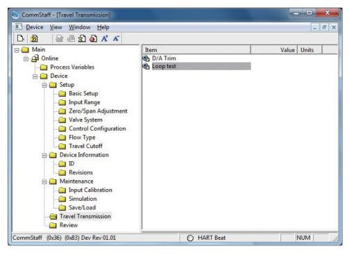
Make sure the loop is set to manual, and configure the dummy output signal in the following window.
