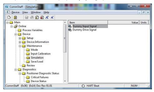
Make sure that the loop is set to manual, and configure the dummy input signal in the window shown below.
