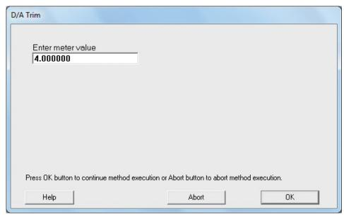
[Note] For ordinary use it is not necessary to execute D/A trim, since it was calibrated before shipment. However, if the actual degree of opening and travel output differ, calibration should be done. In that case, use the following instruments:
