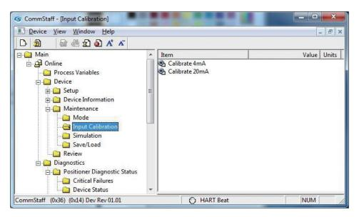
• Set the current input (controller output) to either 4 mA or 20 mA.
