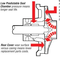
Clearance is set to the rear cover in the shop — not to the casing which is left in the piping.
