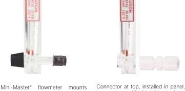
easily from front of panel. Drill two 3/2" or 5/16" dia. holes in panel on 21/16" centers. Insert mounting connector spuds. From rear, slide on the two spring retainers (furnished) and push on rubber or plastic tubing.
