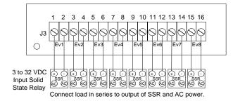
Event Output Option "B" or "K". SSR Model # A007-1732-F4B2 or A007-1732-F4B8 has on board suppression Model # A007-1732-F4K2 or A007-1732-F4K8 has no suppression
