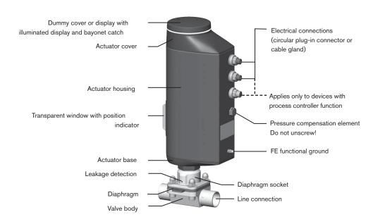
Structure, electromotive diaphragm control valve Type 3363
