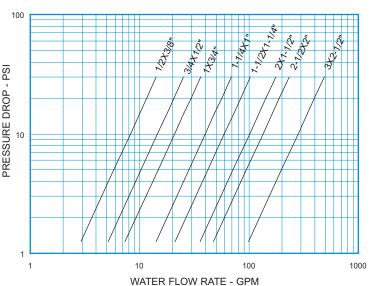
Note: All flow curves and Cv values presume the valves are fully open with 1/2 PSI cracking pressure springs. Consult the factory for more information.
